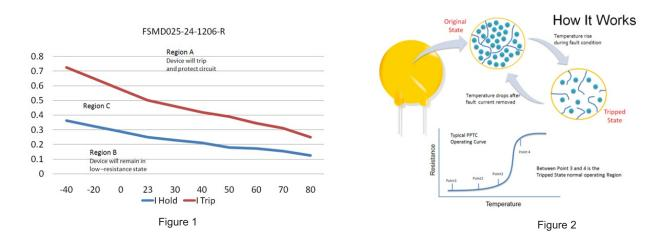
IH (I Hold) defined as the maximum current the device will hold at rated temperature (23°C) without tripping. The probability that the PPTC will trip increases as the current approaches IT (I Trip), defined as the minimum current required to cause the PPTC device to trip at rated temperature.
